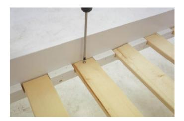
17. Please note not all the slats are required to be fixed to the bed as long as the **top middle and bottom** slats are secured
