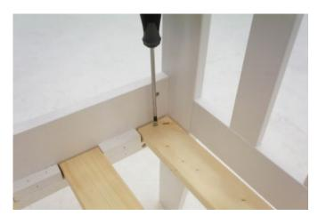
16. To **secure** the frame of the bed in position, ensure you **TIGHTEN** the screws manually located on the slats positioned at the very **top & bottom** ends of the bed and another in the **centre**.
