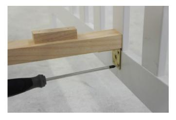
14. Use the small screws in the hardware pack and screw one side of the metal bracket into the footboard and the other side to the bottom end of the centre support rail.
