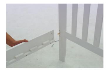
3. Gently raise the bed rail and line it up with the bed head and insert the wooden dowel either on the end of the rail or on the bed head.
