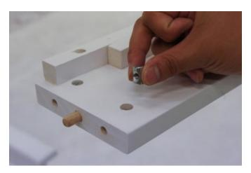
2. Gather the bed rails and at the end of the rail insert the round barrel nut into the 2 holes as shown above, ensuring the hole faces forwards.
